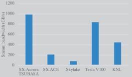
SX-Aurora TSUBASA achieves 4.5, 11.3, 1.2, and 2.2 times higher sustained memory bandwidth than those of SX-ACE, Xeon 6126, Tesla V100, Xeon Phi KNL 7290, respectively. 350 250 200 150 0 SX-Aurora SX-ACE Skylake Tesla V100 KNL TSUBASA
