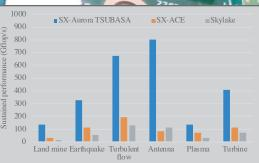
SX-Aurora TSUBASA achieves about 1.97 to 9.75 times faster than SX-ACE due to its high computational capability and high sustained memory bandwidth.
